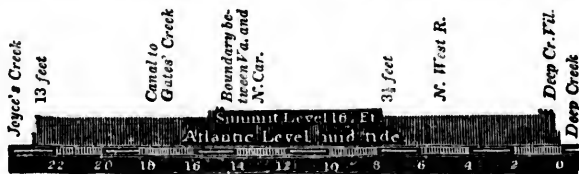
PROFILE VIEW OF THE DISMAL SWAMP CANAL.
